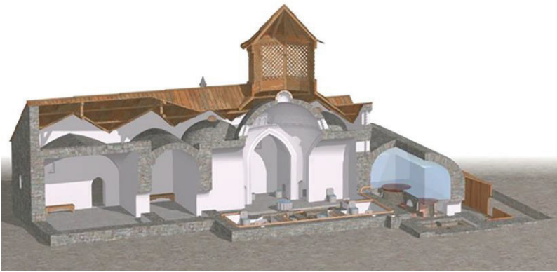
Fig. 5. a. Reconstruction of a public (East Chamber) bathhouse (1260s) of Bolga: layout of the excavated foundation of a public (East Chamber) bathhouse.
