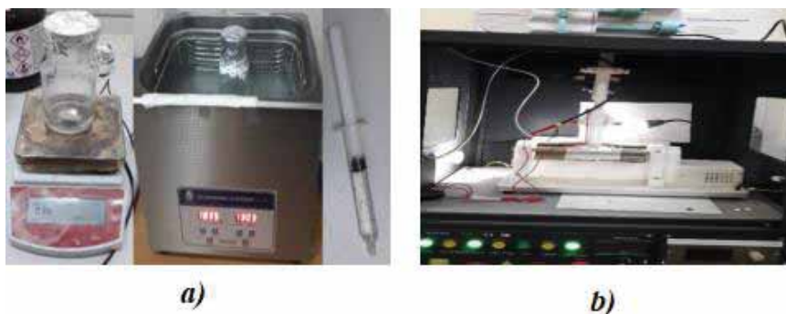
Figure 1. 10 wt,% PVDF-Fe 3 O 4 nanofibrous material preparation steps: a) PVDF solution preparation with hot plate, ultrasonic bath and plastic syringe, b) electrospinning equipment
