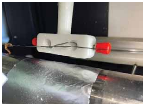
Figure 2. Joining metal bar to the electrospinning equipment
