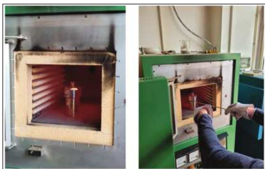
Figure 4. After pyrolyzation process autoclave in muffle and removal of it form muffle.
