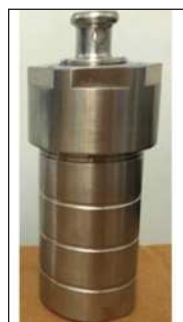
Figure 3. Stainless steel Autoclave.
