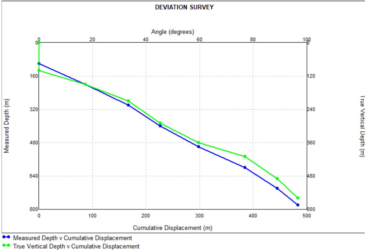
Figure 21. The well profile. The cumulative displacement is shown on the x axis, while the measured depth is shown on the y axis.
