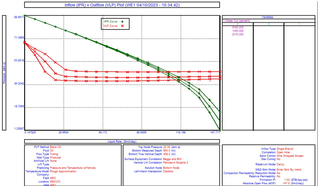
Figure 31. Impacts of increasing water cut on IPR & VLP curves.
