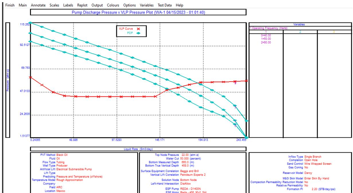
Figure 43. Impacts of different operating frequencies on PDP & VLP curves for ESP.
