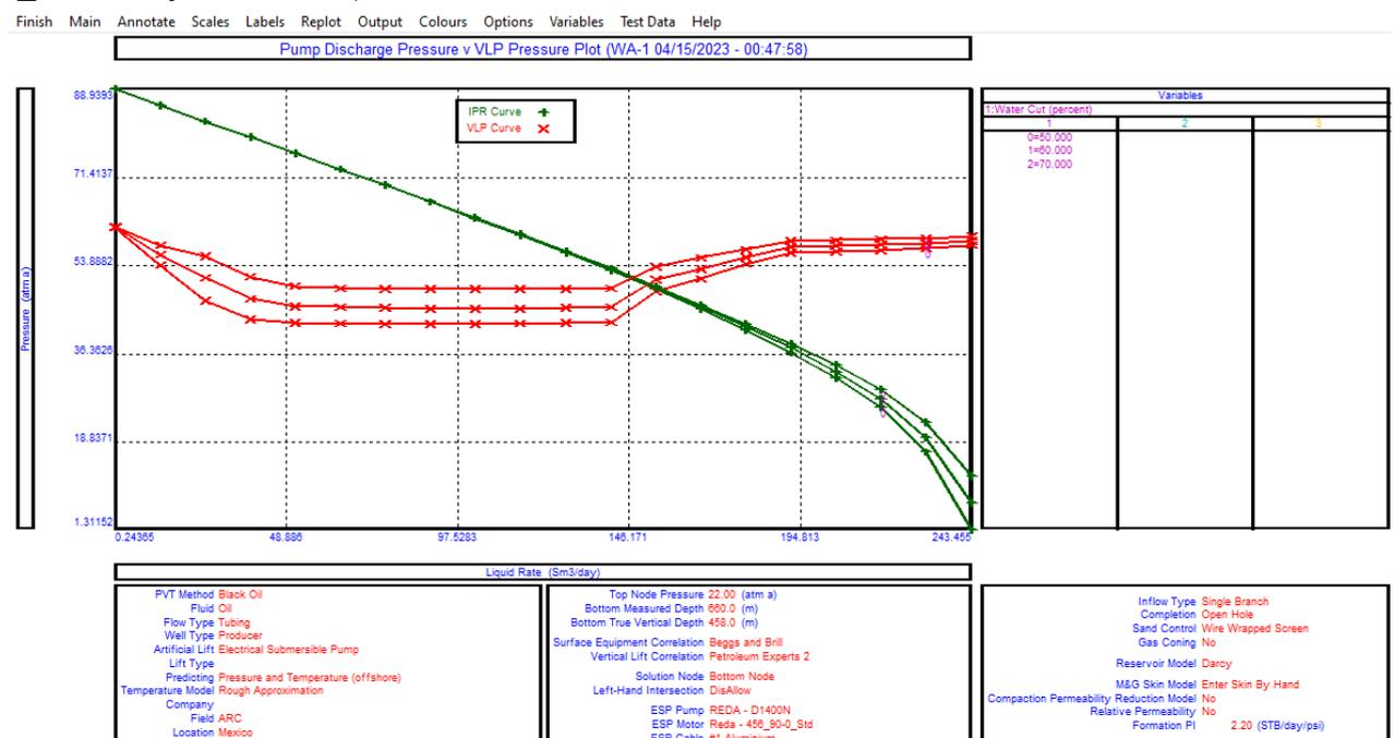
Figure 42.. Impacts of increasing water cut on PDP & VLP curves for ESP
