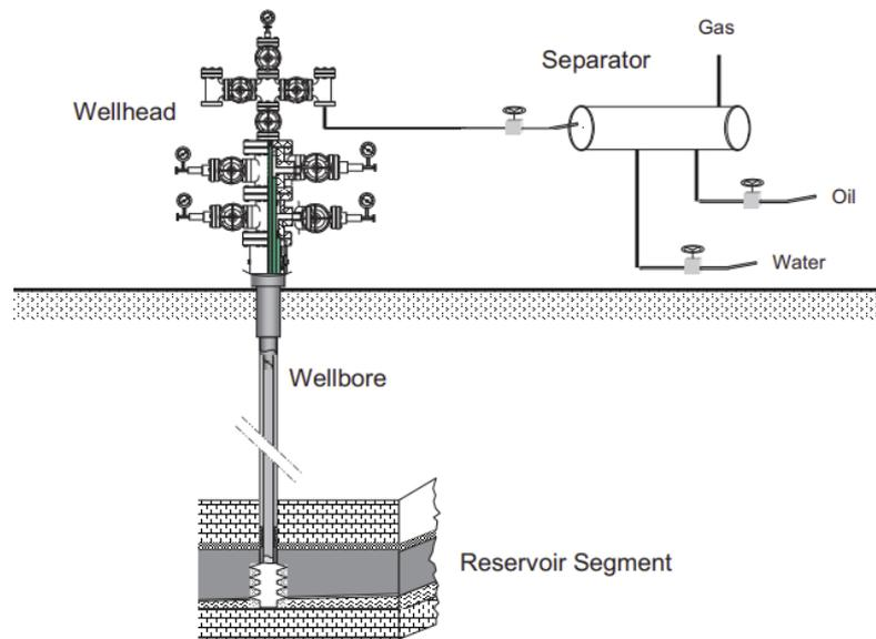
Figure 3. Oil and gas are produced by naturally flowing wells under their own pressure. (2008 by Gulf Publishing Company)
