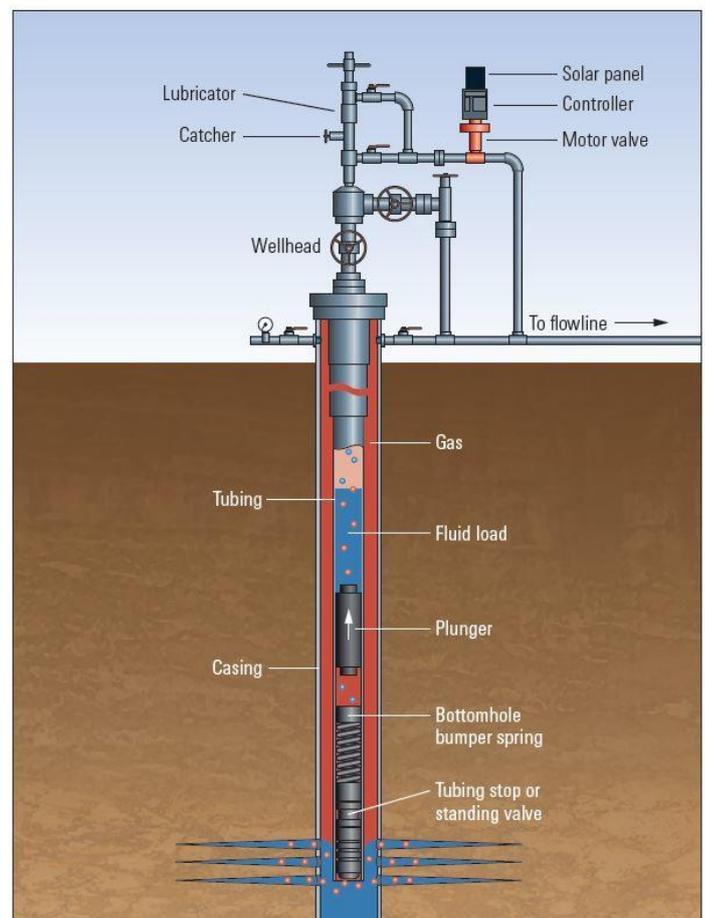
Figure 9. Typical PL configuration (Oilfield Review, 2016).
