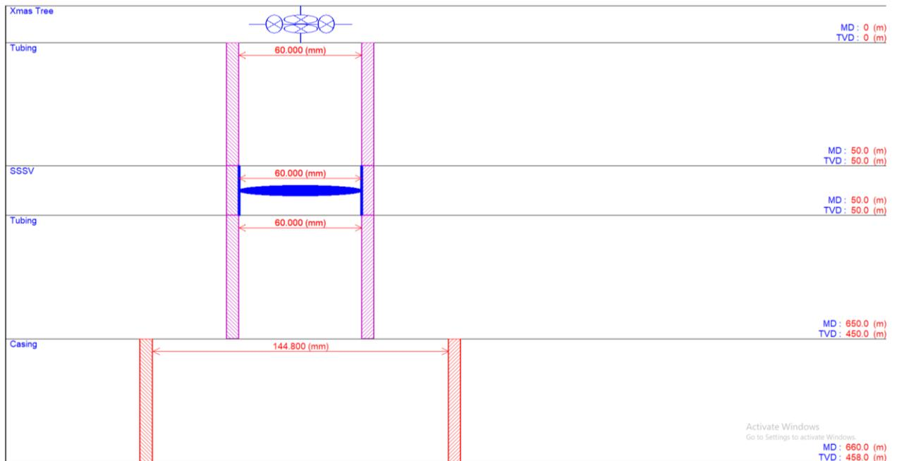
Figure 24. Simple schematic of the downhole equipment
