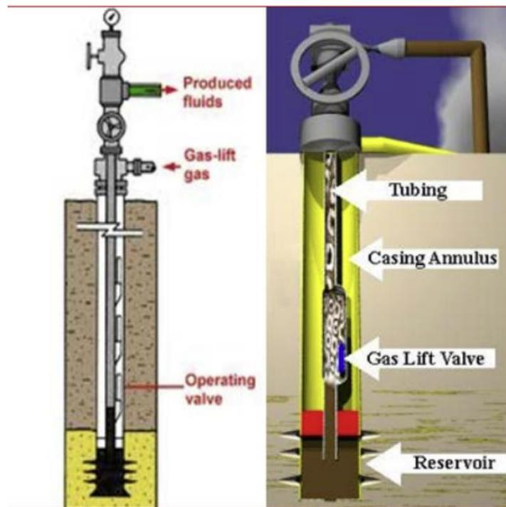
Figure 10. Gas Lift System (Vinegar, 2004)
