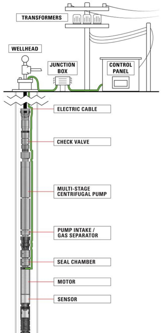
Figure 7. COMPONENTS OF AN ESP SYSTEM. <https://kimray.com/training/how-does-electric-submersible-pump-esp-work>
