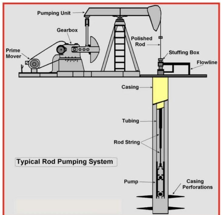
Figure 5. Beam rod pump main components (Di et al. 2018)
