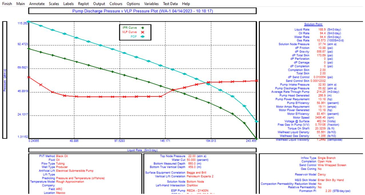
Figure 40. Pump Discharge Pressure vs VLP Plot for ESP-lifted well
