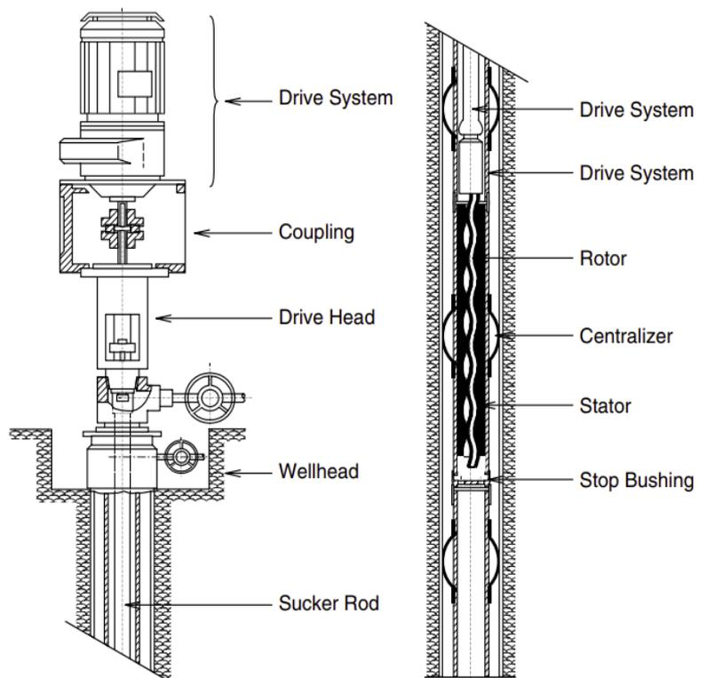
Figure 8. Visualization of a PCP system. *Petroleum Production Engineering, Second Edition*
