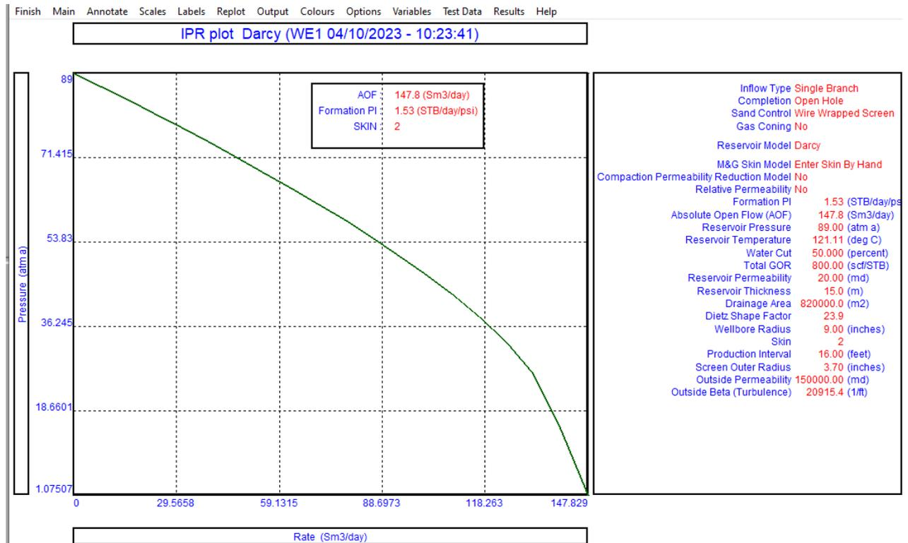
Figure 18. Plot of IPR according to Darcy Reservoir Model.
