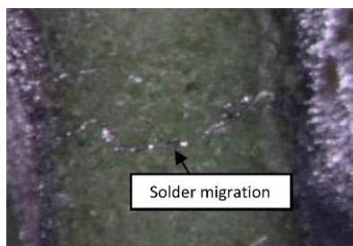
Figure 9. Solder migration between two solder joints
