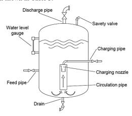
Figure 15. Variable-pressure steam accumulator [17].
