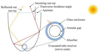
Figure 5. Schematic diagram of a CPC
