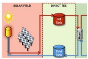
Figure 12. Two-tanks direct TES system integrated into a CSP plant [21]
