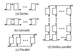
Figure 9. Basic arrangements of banks of solar collectors [12].
