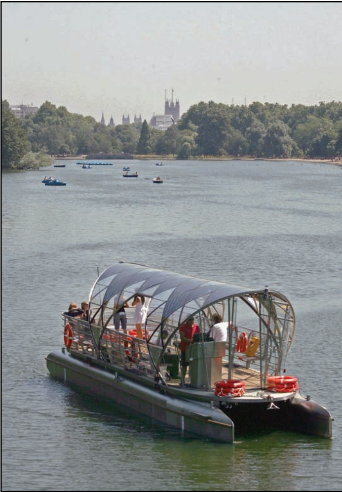
Solar panels on the roof provide the power for this boat, which carries passengers in London, England.
