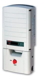
To read the LCD display of your SolarEdge inverter, press the LCD light button located on the bottom of your inverter. If you have an integrated DC disconnect with a red ON/OFF switch on the front, the LCD light button will be located on the bottom of the top part of the inverter, just below the LCD screen.
