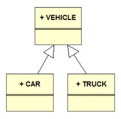
The vehicle class would be the generalisation (super class) and the car and truck classes would be specialisations (sub types).
