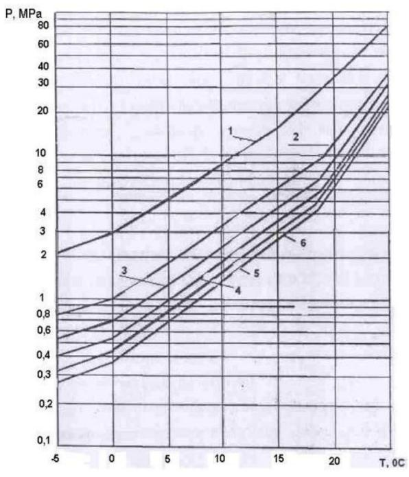
Curves of balance parameters in hidrate generation of natural gases
