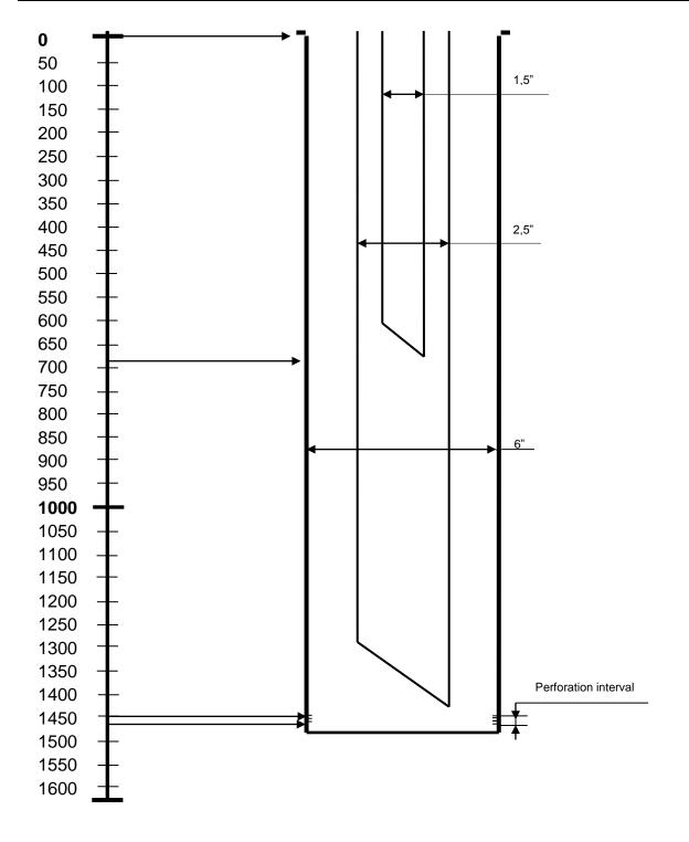
Lets watch water is accumulated to the bottom holeof 1153 numbered well or not:
