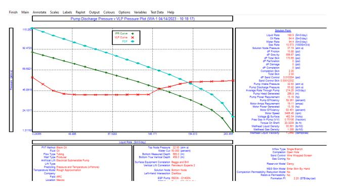
Figure 40.Pump Discharge Pressure vs VLP Plot for ESP-lifted well
