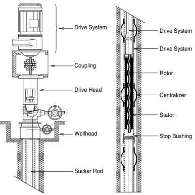
Figure 8.Visualization of a PCP system.Petroleum Production Engineering, Second Edition
