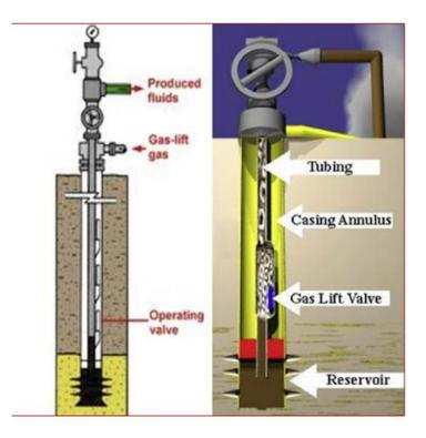
Figure 10.Gas Lift System (Vinegar, 2004)
