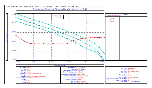
Figure 43.Impacts of different operating frequencies on PDP & VLP curves for ESP.
