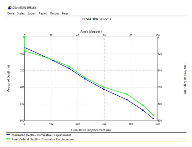
Figure 21. The well profile. The cumulative displacement is shown on the x axis, while the measured depth is shown on the y axis.
