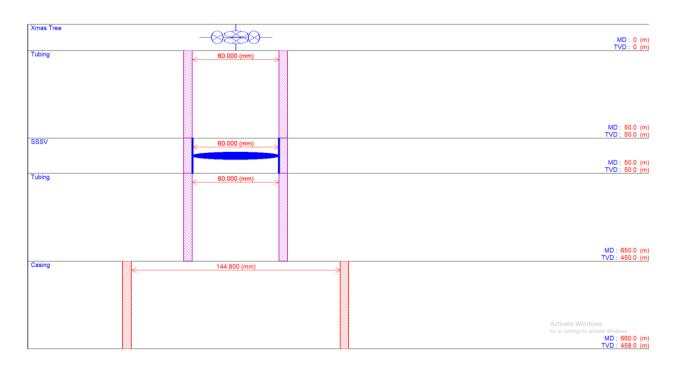
Figure 24.Simple schematic of the downhole equipment
