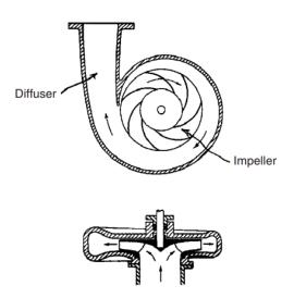
Figure 6. An internal schematic of centrifugal pump. Boyun Guo2007
