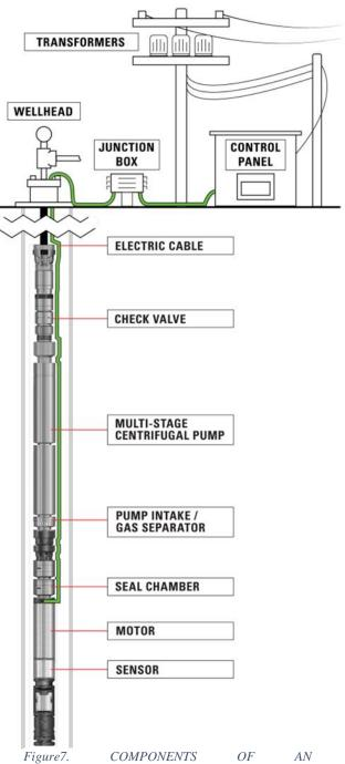
Figure7. COMPONENTS OF AN ESP SYSTEM.https://kimray.com/training/how-does-electricsubmersible-pump-esp-work
