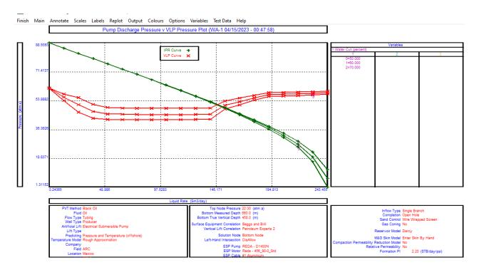
Figure 42.. Impacts of increasing water cut on PDP & VLP curves for ESP
