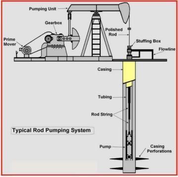
Figure 5.Beam rod pump main components (Di et al. 2018)
