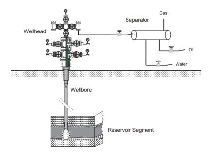
Figure 3.0il and gas are produced by naturally flowing wells under their own pressure. (2008 by Gulf Publishing Company)
