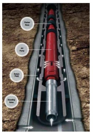
*Figure 7. Jet pump (Pugh, 2009).Overview of Hydraulic Pumping (Jet and Piston). Weatherford CP.*
