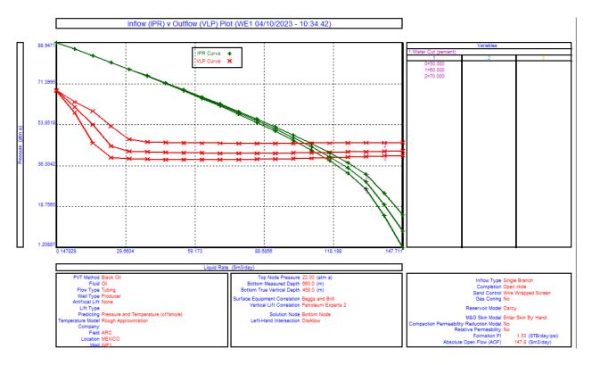
Figure 31.Impacts of increasing water cut on IPR & VLP curves.
