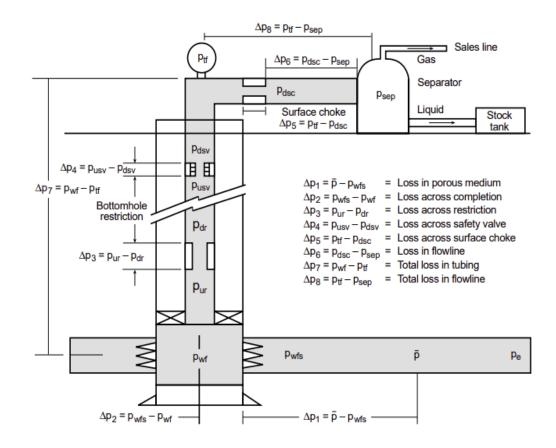
Figure 2.Pressure losses along the system Pdr = downstream restriction pressure, Pdsc = pressure downstream of the surface choke, Pdsv = pressure downstream of the safety valve, Psep = separator pressure, Ptf = tubing flowing pressure, pur = upstream restriction pressure, Pusv = pressure upstream of the safety valve, Pwfs = wellbore sandface pressure (Economides & Nolte, 2000).
