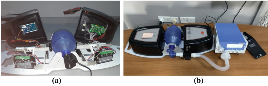
Fig. 1. The designed AMVS. (a) electronic parts, (b) AMVS with artificial lung
