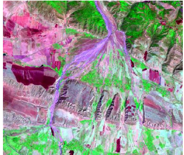
Fig. 3. Bands 742 (RGB) of Landsat 7. Stream appears to be flowing through a small shutter ridge, which is formed by parallel strands of major strike-slip fault. Image is approximately 17 km across. Located along the proposed Baku-Ceyhan pipeline route.
