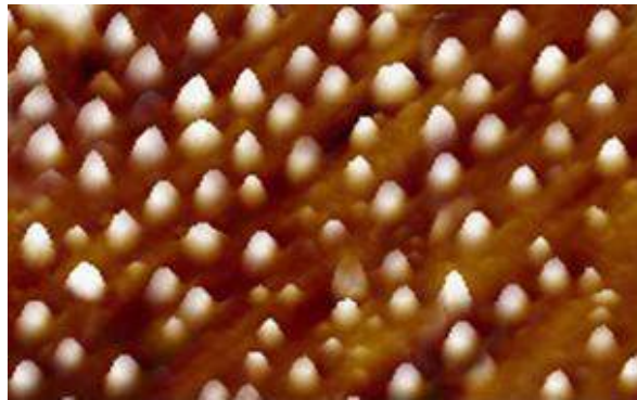
Fig.2. AFM-images Bi_2Te_3<Se> , NI are ordered formed nano-islands on the places of dislocations on surface (0001).
