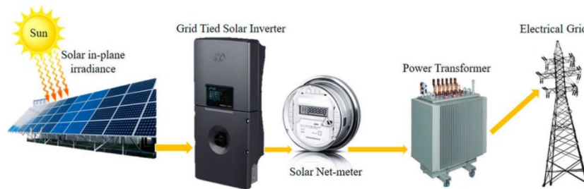
Figure 7. Schematic of the simulated solar power plant
