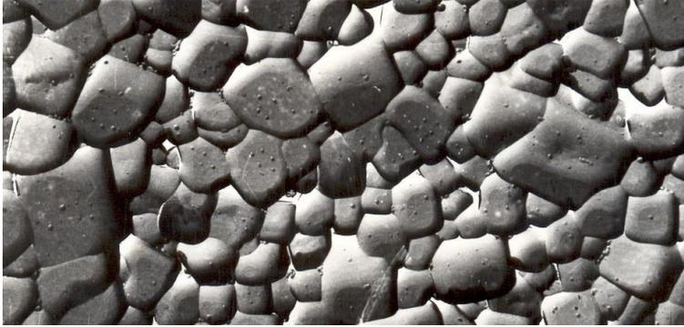
**Figure 5.** Microcrystalline structure of  $\text{Bi}_2\text{Te}_3$  hexagonal phase.
