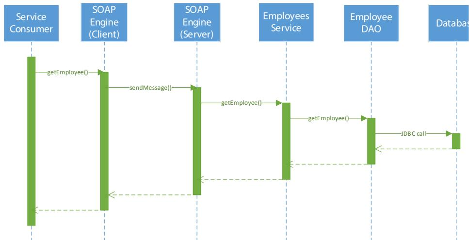
**Figure 4-3.** Sequence diagram of a *getEmployee* operation
