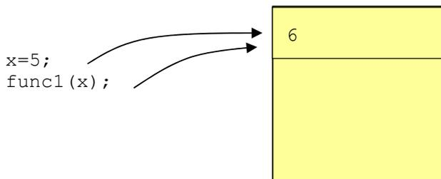
Defining a function parameter as reference parameter is made by placing an `&` character after the data type:
