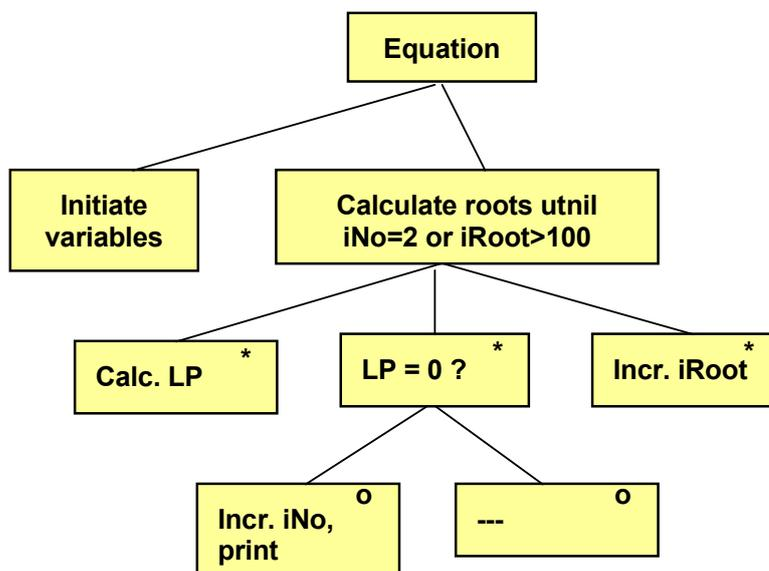
The variable `iNo` is used to count the number of roots to the equation that we have got. The variable `iRoot` is the x value in the equation which in each loop turn is used to calculate LP. The value of `iRoot` starts with 1 and is increased by 1 for each loop turn. If the value of `LP = 0`, we increase the value of `iNo` and print the root (x value).
