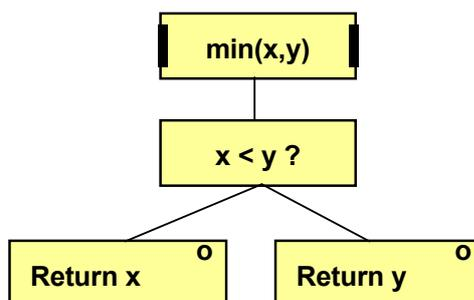
As shown by the JSP the function takes two parameters, x and y, and checks whether x is less than y. If so, x is returned, otherwise y.
