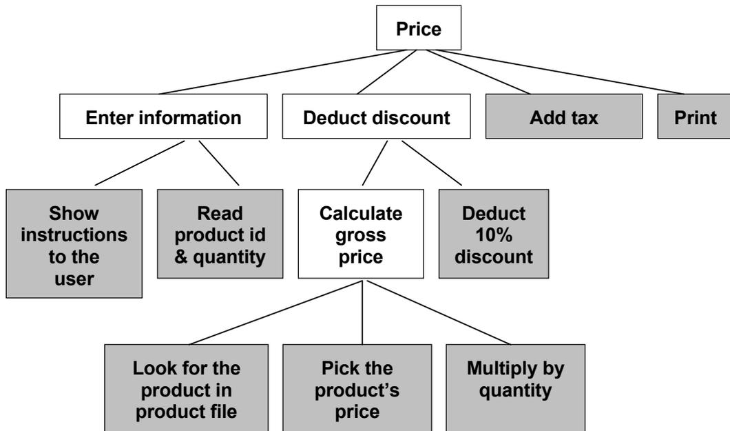
We could refine the algorithm further, but let us say that we are satisfied with the detail level. The shadowed boxes in the graph are the end points at the lowest level, the "leaves of the tree". These are the boxes to be used for coding, from left to right.
