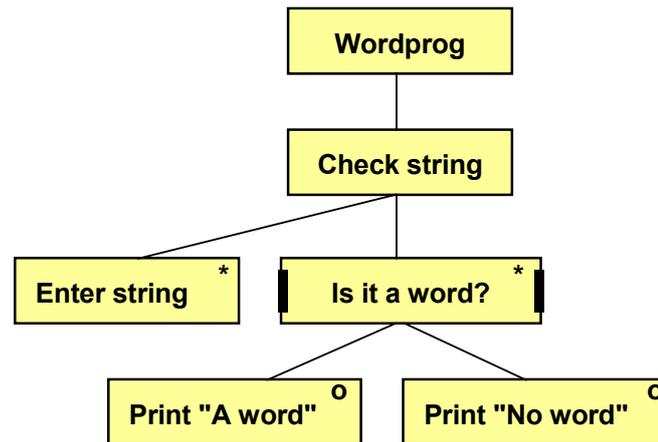
The program has a loop 'Check string'. For each turn of the loop we read a string from the keyboard. The string is sent to the function `word()`. If 1 is returned by the function, we print 'A word'. If 0 is returned, we print 'No word'.
