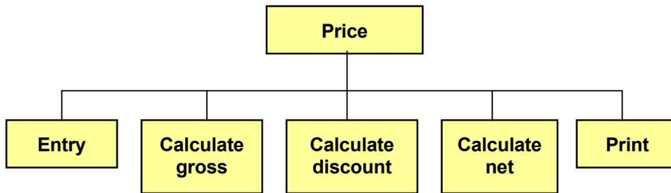
All boxes except “Calculate discount” are rather simple to code. “Calculate discount” requires a closer examination. It has a condition included which says that the discount is different depending on whether gross is less or greater than 500. We’ll break down that box:
