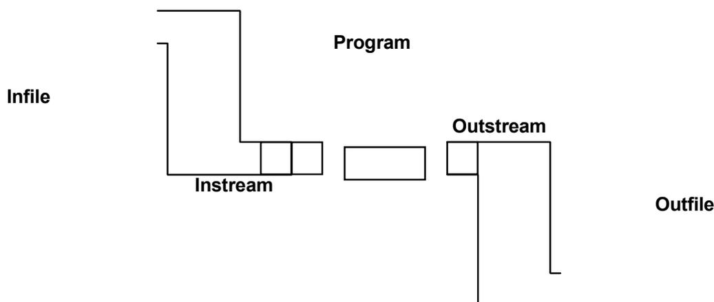
When data is to be read from a disk file (infile) to a program, it goes via an intermediary store (instream) which works as a buffer between the hard disk and the program, where data is queued to be read to the program.
