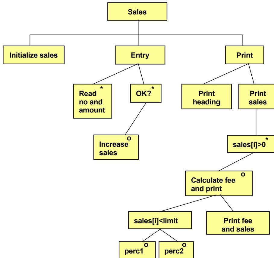
If the sales amount is below the limit 50000:- the lower percent 10% will be applied. Otherwise the greater percent 15% will be applied to the exceeding amount. When the fee calculation is finished, the fee and sales amount are printed.
