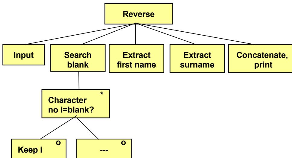
First we read the name from the user input. Then we search for the position of the blank by looping through the characters and checking if any of them is blank. When a blank is found we save its position.
