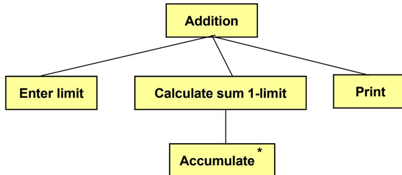
First the user is prompted for a limit. The following loop goes from 1 to limit with the loop variable  $i$ . For each turn of the loop we add the value of  $i$  to the sum, i.e. we accumulate the numbers. Finally we print the accumulated sum. Note that the operation to be repeated (Accumulate) in the loop is indicated by an asterisk in the JSP graph.
