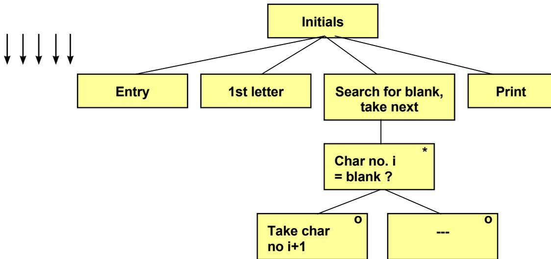
Searching for the blank is made in a loop. For each turn of the loop we check if character no. i is blank. If so, we take character no. i+1 as the second initial. Here is the code:
