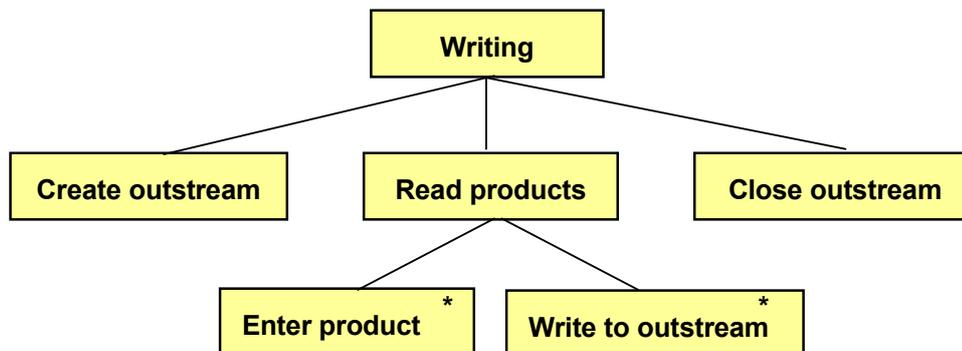
First we declare an ostream and attach it to the file `prodfile.txt`. Entry of product names from the keyboard is made in a loop. As soon as a product name has been entered by the user, it is written to the ostream. At entry completion, we close the ostream.
