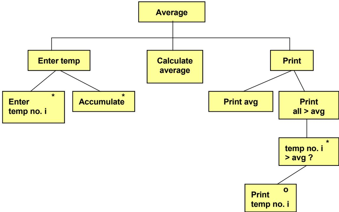
The average calculation is simple. We don't have to detail it. However the output is a little more complicated. First we print the calculated average. Then we write a loop which in turn checks each item of the array against the calculated average. If temperature number *i* is greater than the average, we print temp no. *i*.
