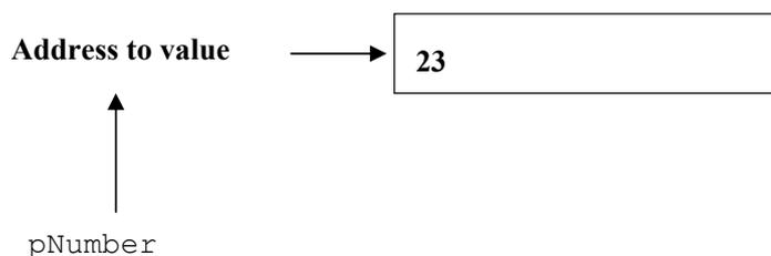
In the figure above we have a pointer named `pNumber`. It contains an address in the primary memory. If we go to that address, there is a number, 23 in our example.
