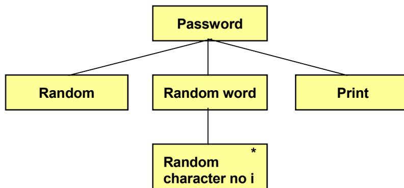
We begin with creating a random length of the password, which we in this example will limit to between 5-7 characters. Then we create as many characters in the interval A-Z (character codes 65-90). The password is then printed. Here is the code:
