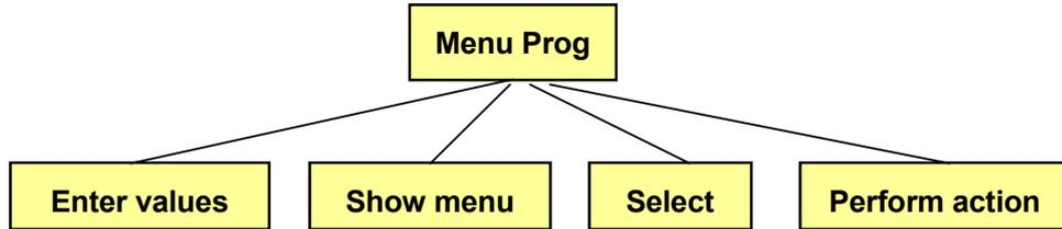
First, the user enters two numbers. Then the menu is displayed on the screen and the user selects an option. Finally the requested action is performed.
