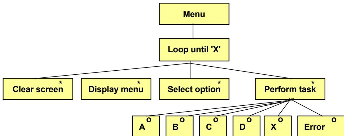
We complete the menu with still another option, X – Exit. As long as the user does not enter X, the loop proceeds. Furthermore we also clean the screen before the menu is displayed, which is the first operation of the loop. Here is the code:
