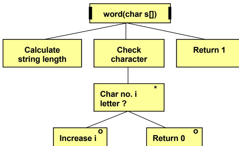
The function begins by calculating the string length. The loop 'Check character' goes through character by character and checks if it is in the interval a-z or A-Z. If so, we increase the loop counter i by 1. Otherwise we return the value 0 and the function is terminated. If all characters are letters, the loop will complete and we return 1.
