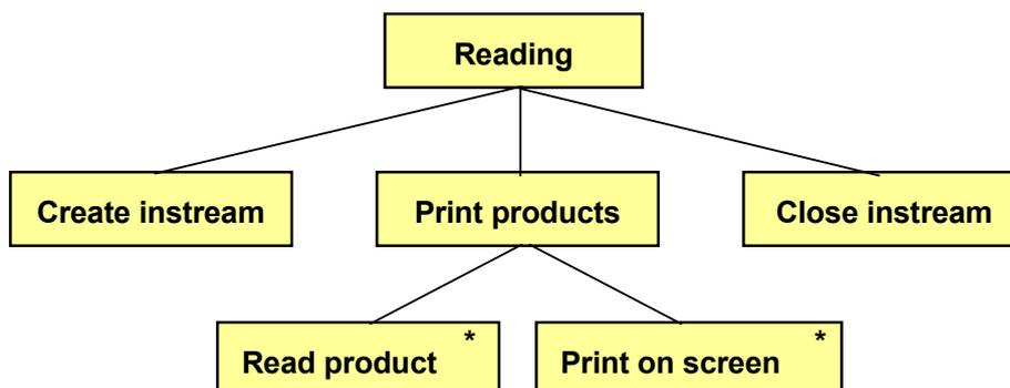
First we declare the instream and attach it to the prodfile.txt file. Reading and printing on the screen is made in a loop where we read one product at a time from the instream and print it on the screen. At completion, we close the instream.
