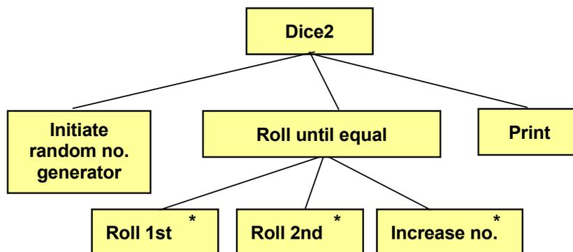
When having initiated the random number generator to a random start position, the loop begins. For each turn, we roll the 1<sup>st</sup> and then the 2<sup>nd</sup> dice, and then increase the counter by 1. When the two rolls are equal the loop is terminated and the number of “double” rolls is printed. Here is the code:
