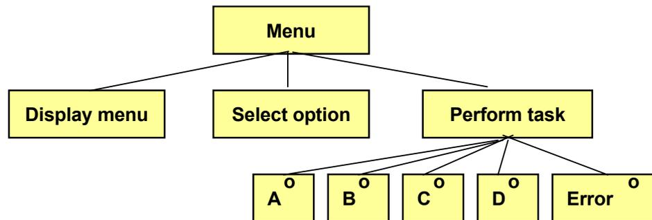
The first action is that the menu is displayed. Then the user is prompted for a choice by means of the letters A-D. Finally the requested option is executed, i.e. a simple text message will be printed. If the user enters another character than A-D, an error message is printed. Here is the code:
