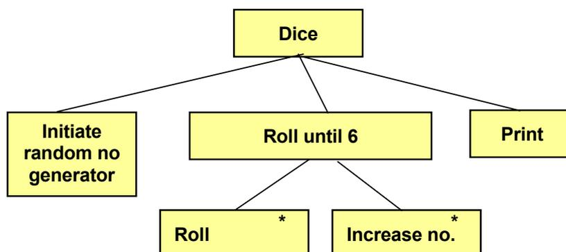
We begin with initiating the random number generator to a randomly selected start position. Then the loop is repeated until we get 6. For each turn of the loop we roll the dice once more and increase the number of rolls by 1. When 6 has been achieved, the loop is terminated and the number of rolls is printed. Here's the code:
