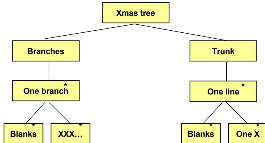
The JSP graph tells us that there is one outer loop for the branches, where each turn of the loop prints a branch. We then have one inner loop that prints the correct number of blanks and one inner loop that prints the 'X's. The same is true for the trunk where we have an outer loop where each turn of the loop prints one line of the trunk, and one inner loop that prints the blanks before one single 'X' is printed. The code is as follows:
