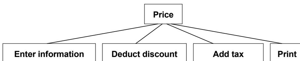
The upper box is the name of the program. We have split the solution into four steps at an overview level. You read the steps from left to right. As you probably realize the algorithm is too rough to be able to write code. So we proceed by refining the solution to the next level:
