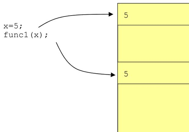
The variable `x` has the value 5 stored in a memory location. When `func1()` is called, that value is copied to another memory location used by the function. If a statement in the function would change the value to 6, the memory location of the function is affected, but not the original value of `x`:
