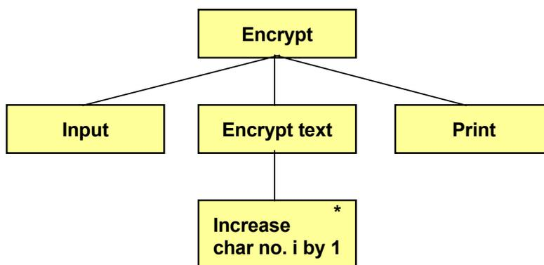
The user is first prompted for a text. The encryption takes character by character from the string array and increases the character code by 1. Finally we print the encrypted message. Here is the code:
