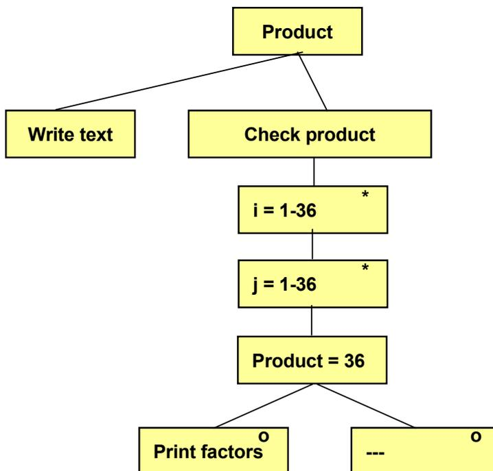
Under “Check product” we have an outer loop with the loop variable `i` and an inner loop with loop variable `j`. Inside the loop we check if the product of `i` and `j` makes 36. If so, `i` and `j` are printed.
