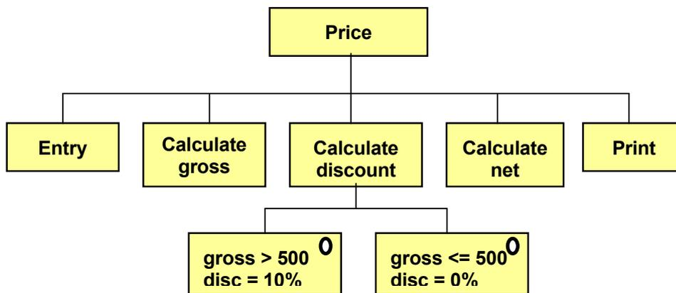
A conditional situation in JSP is identified by a ring in the upper right corner of the box. That implies that only one of the boxes will be executed. Here is the code:
