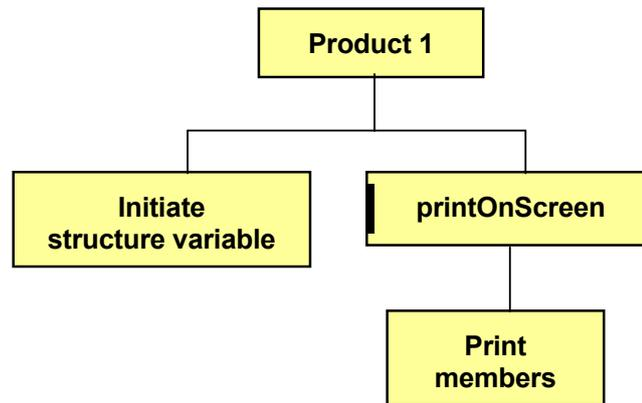
We initiate a structure variable, which is sent to the function, where the members are printed.
