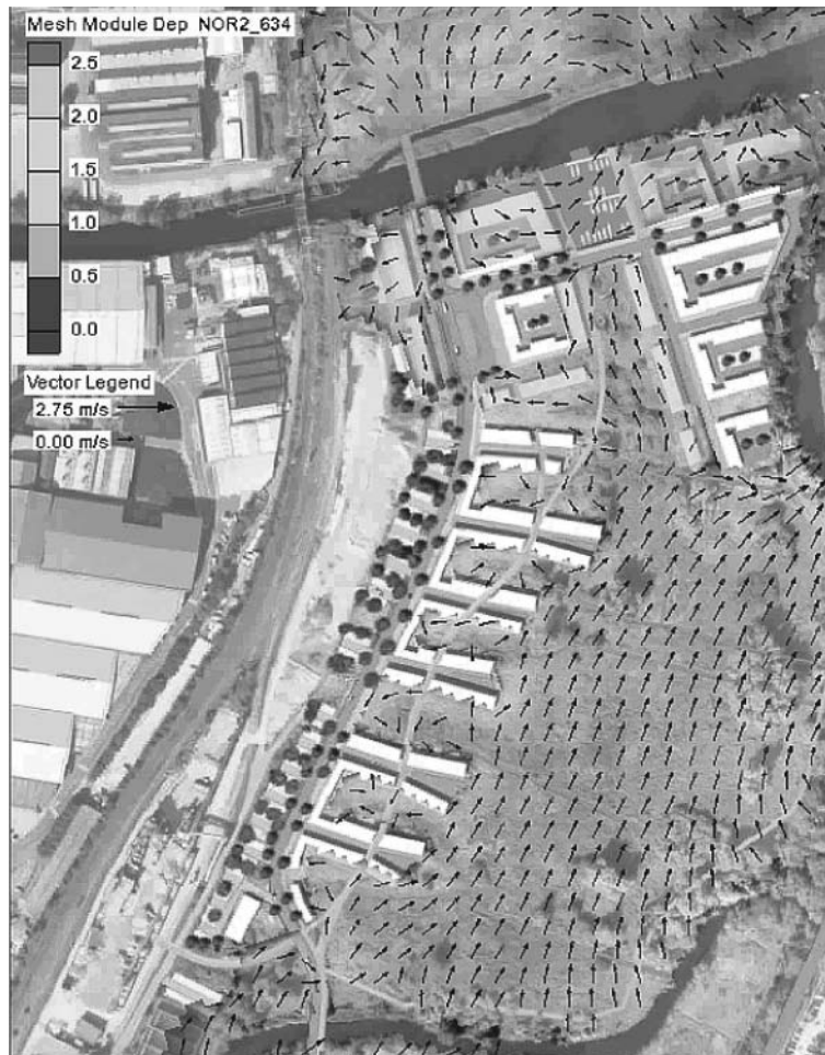
Figure 5.8: Extracted images from an animation of a 1 in 1000 year flood on a new development plan in Norwich, UK. Source: JBA Consulting and Baca Architects
