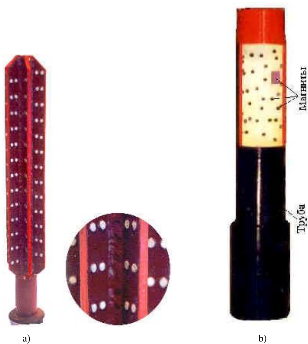
Figure 4. General view of the magnetic treatment of liquid systems УМЖ-122 (a) and УМЖ-73-005 (b).[1]
